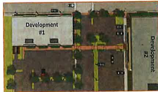
This illustration shows two developments on adjoining lots sharing parking and an access drive. A sidewalk connects the two developments through the parking area.
