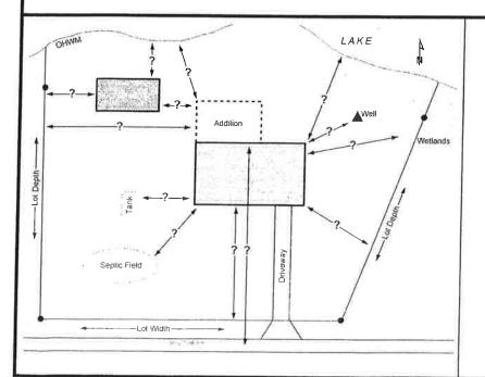
Site plans must be drawn to scale and/or all dimensions given, such as: Location and dimensions of the project Location and dimensions of existing structures Dimensions of the property Location and names of abutting roads, lakes & **Streams** North arrow Owner's name
