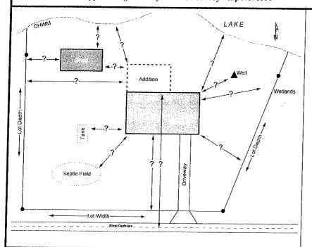
Site plans must be drawn to scale and/or all dimensions given, such as: Location and dimensions of the project Location and dimensions of existing structures Dimensions of the property Location and names of abutting roads, lakes & **Streams**
